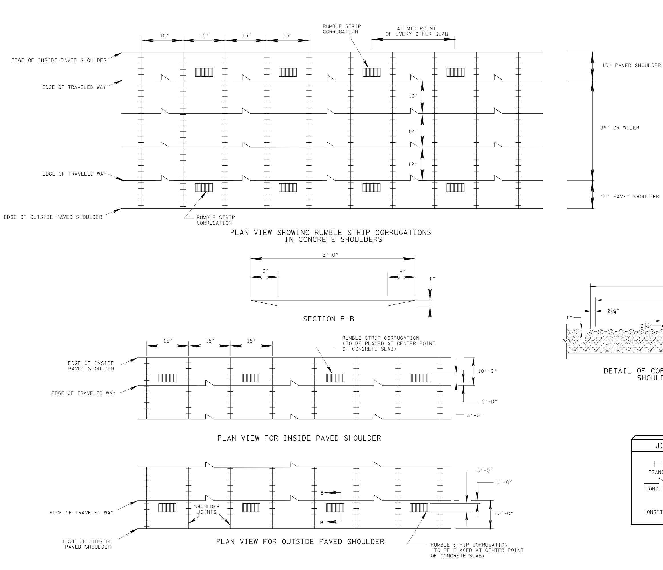
REV. 5-27-01: CHANGED VARIABLE JOINT SPACING TO 15' CONSTANT IN ALL VIEWS TO MATCH STD. DWG. NO. RP-J-1.
